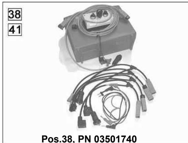
Solenoid valve test set, Hako spare parts number 03501740, for testing the power supply, the current and the resistance of solenoid valves.
